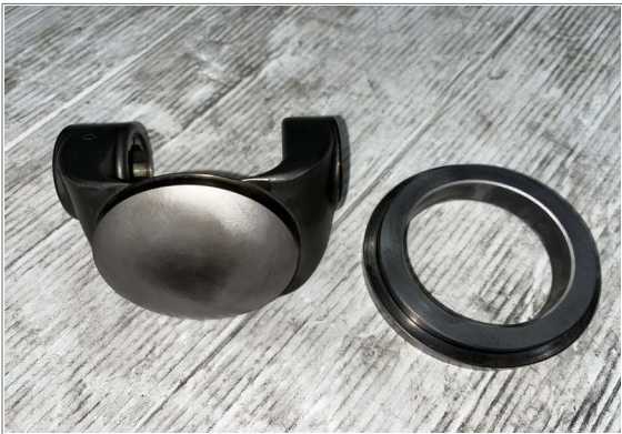
A condition of plug-seat are good after clean & laping.
