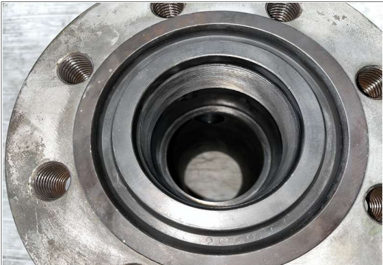
A condition of valve body after clean.
