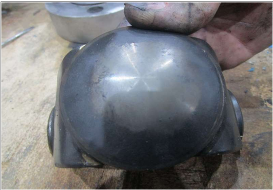
A condition of plug-seat before clean & laping.
